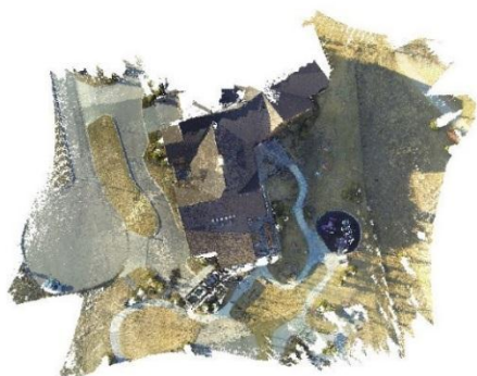
Figure 6. Dense image-based point cloud derived from the UAV image dataset after applying the proposed disparity refinement
